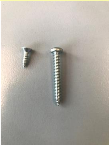
Figure 15: Screws for changing the tension.
