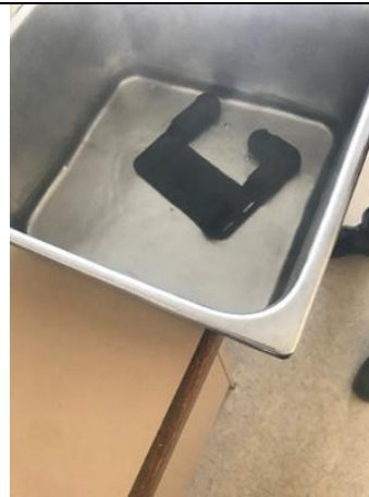
Figure 10: Softening cuff with hot water to mould it. Possible due to PLA filament choice.
