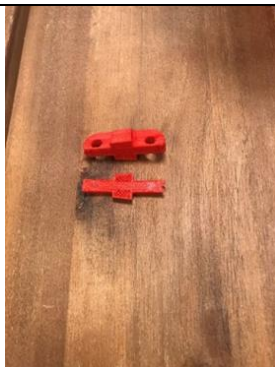
Figure 5: Broken fingertip – wrong density and layer, weakness.
